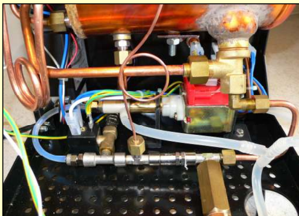
Brew water path, with de-aerator, solenoid valve and OPV assembly, all easy to reach
