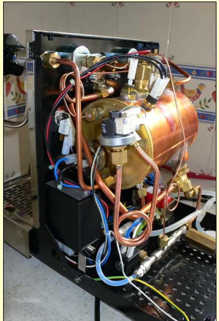
Removal of the outer case, gives easy access to all components, e.g. heating element.
