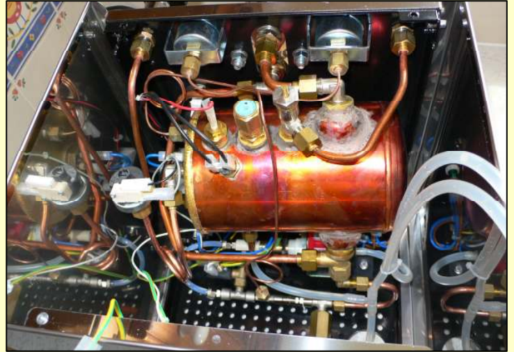
The powerhouse of the machine accessible from the top, with the removal of only 4 screws
