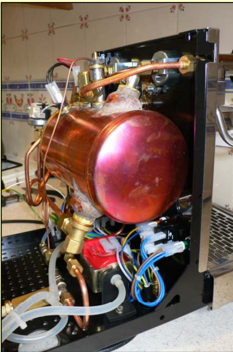
The vibe pump tucked under the boiler
