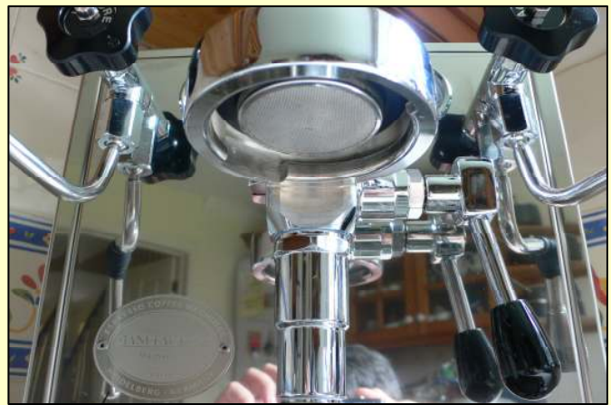
The beautiful lever operated E61 group, just waiting to make that espresso or latte!
