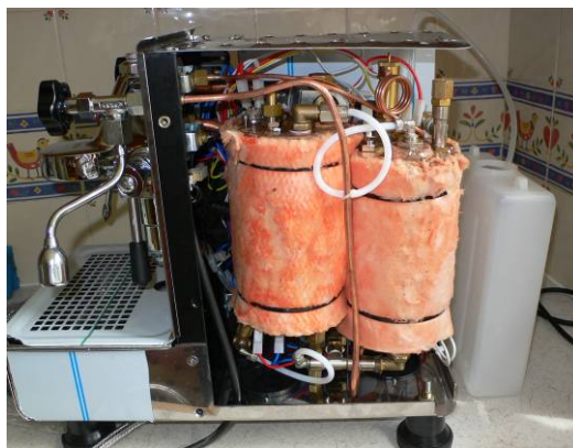
The twin boilers and water tank (removed)
