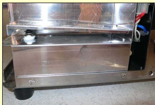
I admire the simplicity of the water tank level sensor. A mechanically very simple, effective and reliable system of a; flap, switch and single spring!
