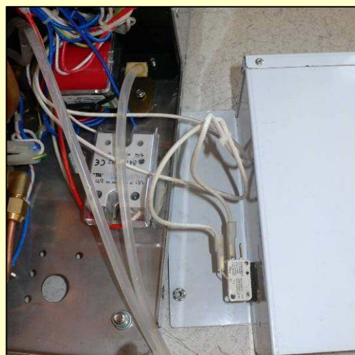
Reliable, easy to replace and low cost Vibration pump, plus SSR relay for noiseless brew boiler heating element operation. The 25 amp shielded SSR is particularly well heat sunk
