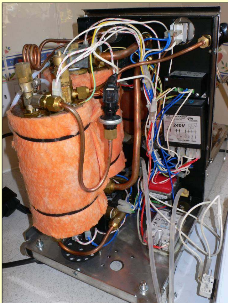
Large 12mm diameter thermosyphon pipes. Nice quality braided wiring, very easy access for maintenance.
