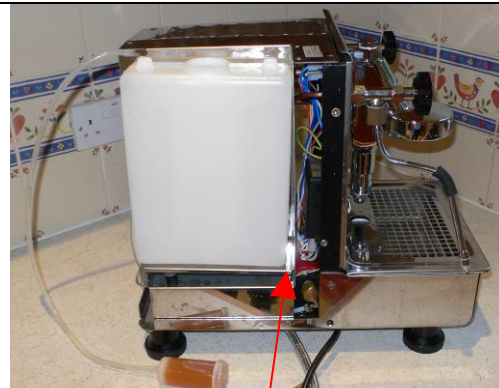
A shot with the case removed but the water tank in place, note the simple rocker platform
