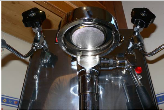
The group from the bottom, all standard 58mm, E61 , water and steam wands on ball joints
