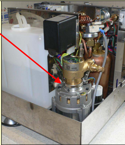
Rotary pump is now vertical & rubber mounted, which reduces vibration considerably and allowed the twin boilers to be fitted in the same case.
