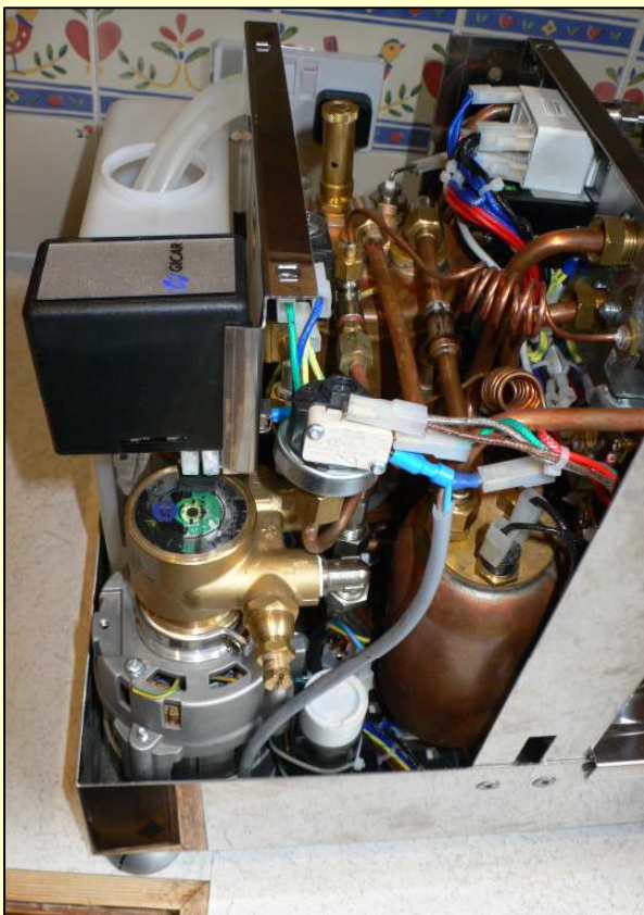
The rotary pump and powerhouse of a motor, plus a good view of the nicely made 0.8l brew boiler. Please ignore the grey lead; it's my own modification to test switching the steam boiler independently
