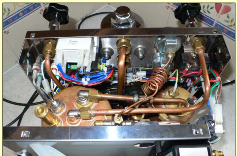
On the left the Gicar PID and heavy duty relay, on the right the Solid state switch
