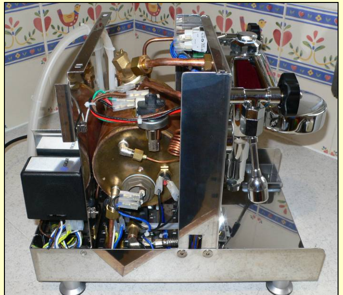
Removal of the outer case, gives easy access to all components, e.g. heating element.
