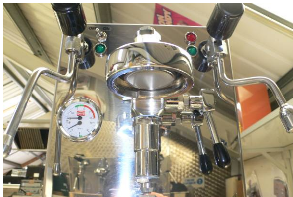
The group, steam and water wands from below (note the ball joint mountings for the wands)
